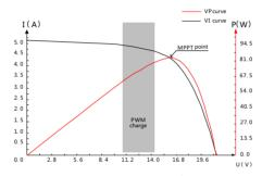
Fig.1-2 Output Characteristic Curve for Solar Battery
