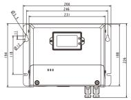
Product size: 266\*226\*119mm Installation size: 246\*118mm Fixing hole position: Φ5.5mm Wire specification: 20-2AWG
