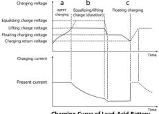
Charging Curve of Lead-Acid Battery
