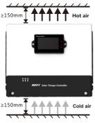
Fig. 2.1 Installation and Heat Dissipation
