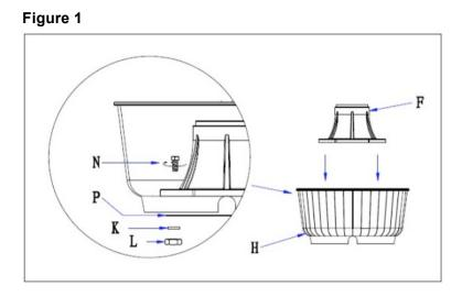
(SEE FIGURE 1) Attach lamp post base (F) to Bottom planter base (H) using M10 bolts (N), mounting plate (P), Flat washer (K) and hex Nut (L). Make sure the mounting plate, flat washer and hex nut are secured to the hex bolt on the underside of the bottom of the planter base (H).
